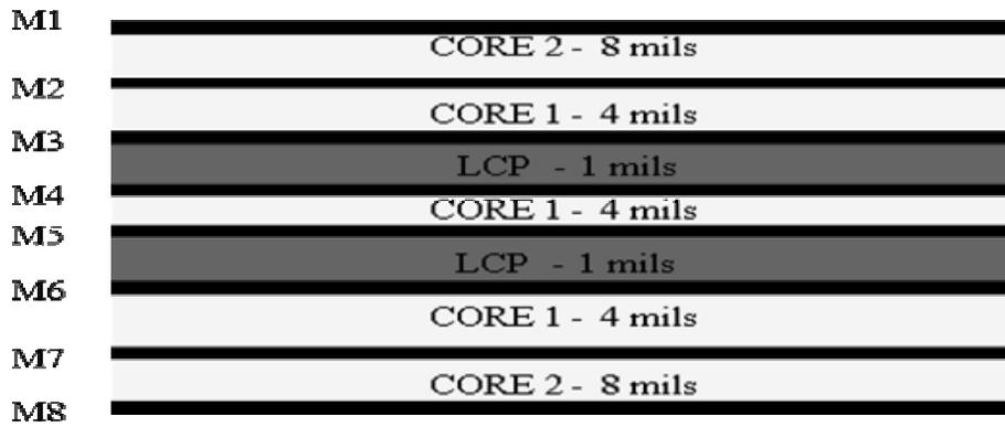
Figure 4.1. Cross-section of the balanced-LCP substrate
