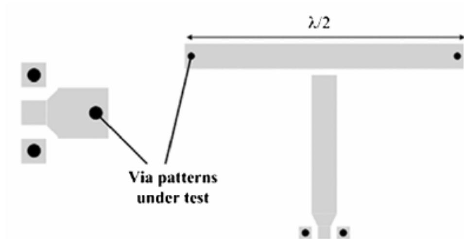
Figure 1.5. T-resonator for characterizing single via
