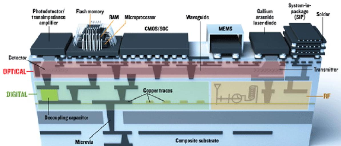
Figure 1.2. The state-of-the-art mixed-signal SOP technology [10]
