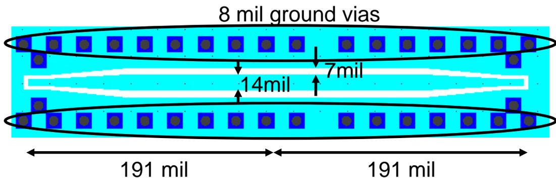
Figure 3.4. The layout of the through standard
