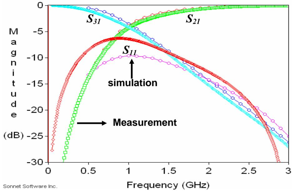
Figure 5.14. Measured S parameter results of IF balun
