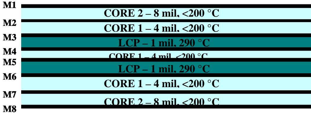
Figure 2.4. Cross-section of two-layer balanced LCP substrate with melt temperature
