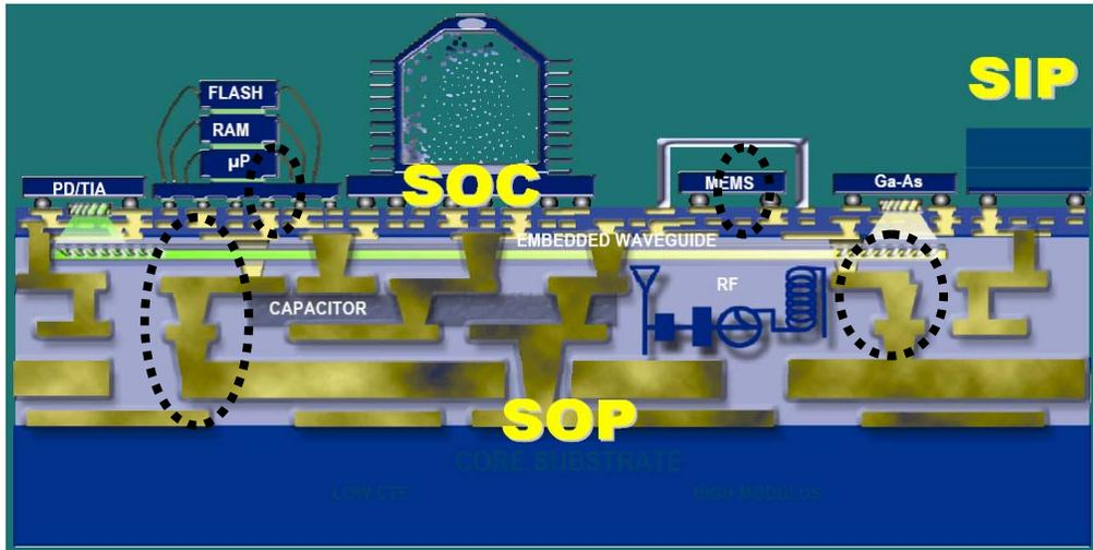
Figure 3.1. Vertical interconnects in 3D integration using SOP
