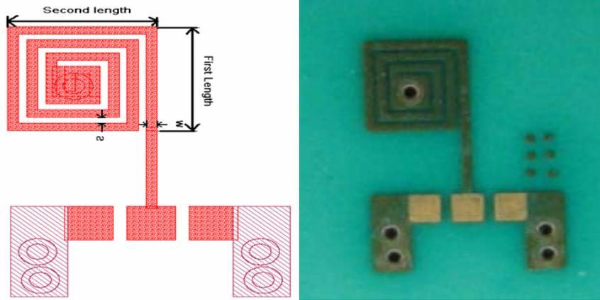
Figure 4.2. Layout and photograph of the designed inductor
