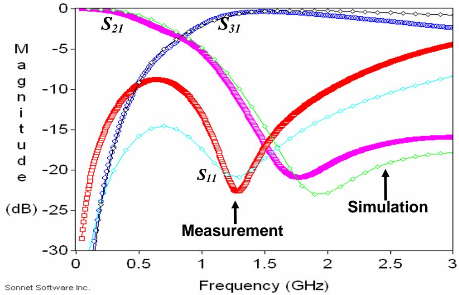
Figure 5.13. Measured S parameter results of LO balun
