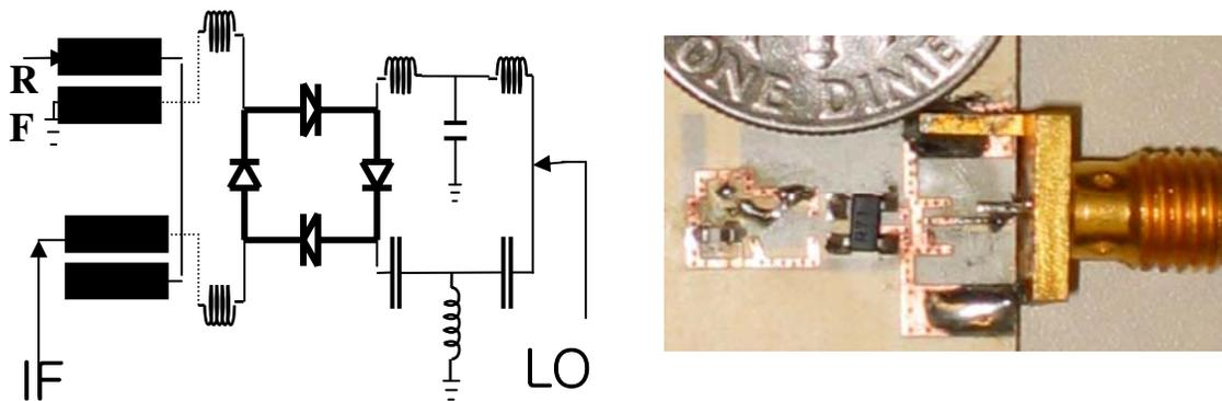
Figure 5.7. Double balanced mixer: schematic and photograph
