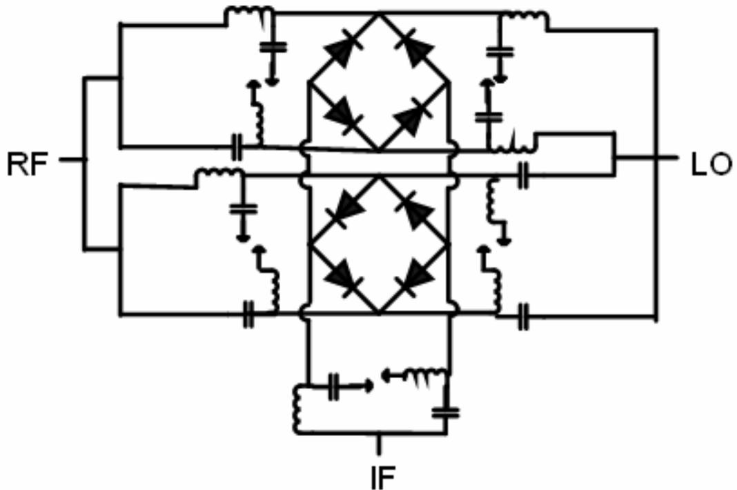
Figure 5.12. Schematic of a double doubly balanced mixer [63]
