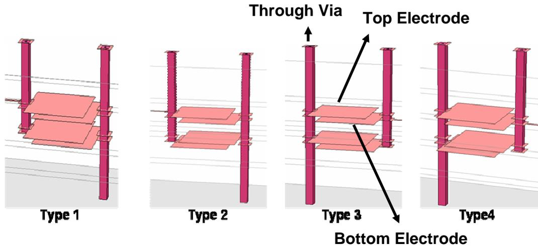
Figure 4.15. 3D layout of the four types of 3D capacitors
