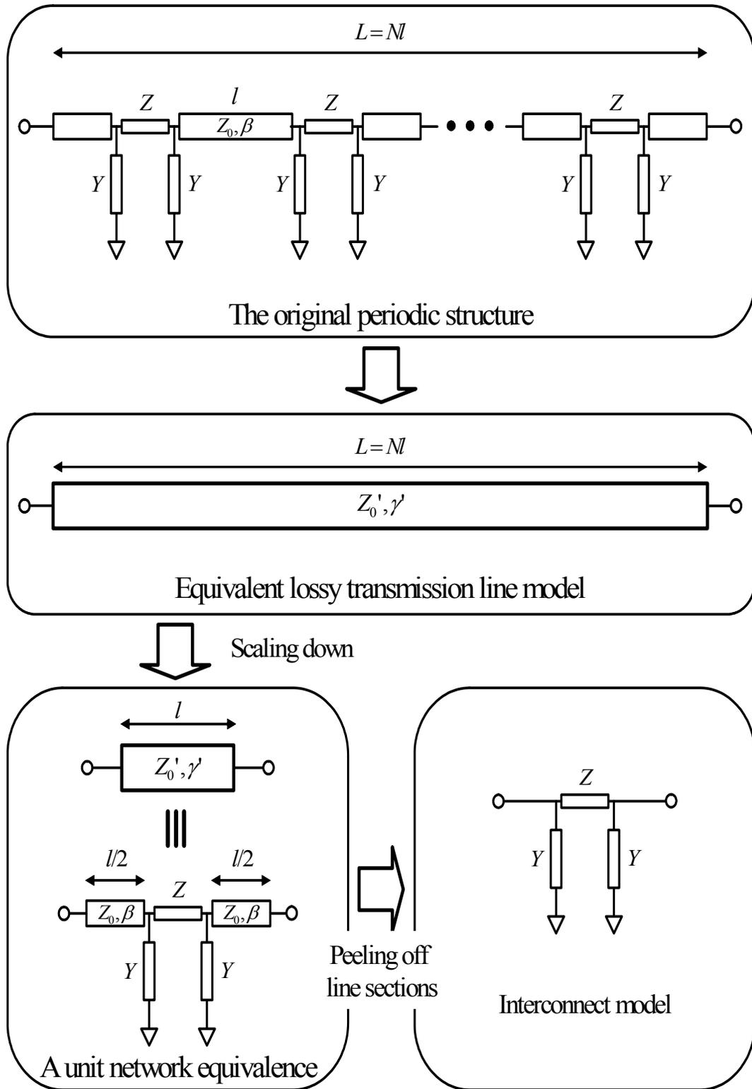
Figure 3.3. The procedure for characterizing vertical interconnect
