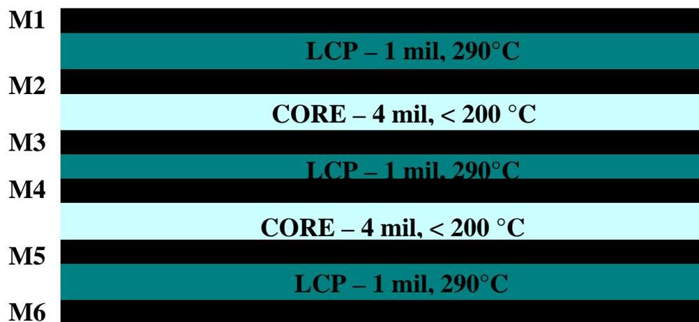
Figure 2.2. Cross-section of the inhomogeneous three-layer LCP substrate with melt temperatures
