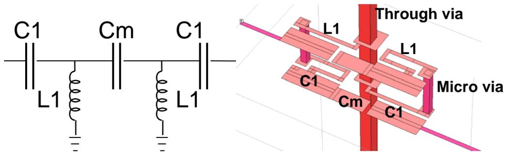
Figure 5.3. Schematic and layout of the designed filter
