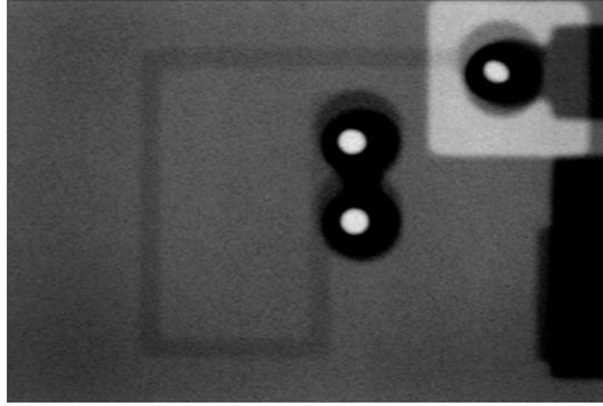
Figure 4.6. X-ray of Inductor 3 in TV2
