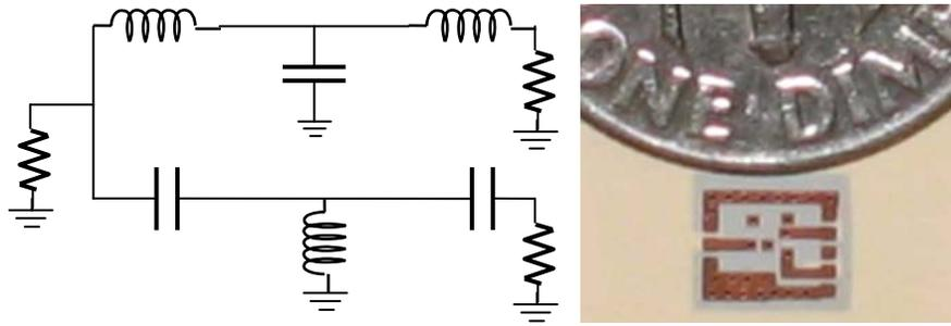
Figure 5.5. Schematic and photograph of a lumped balun
