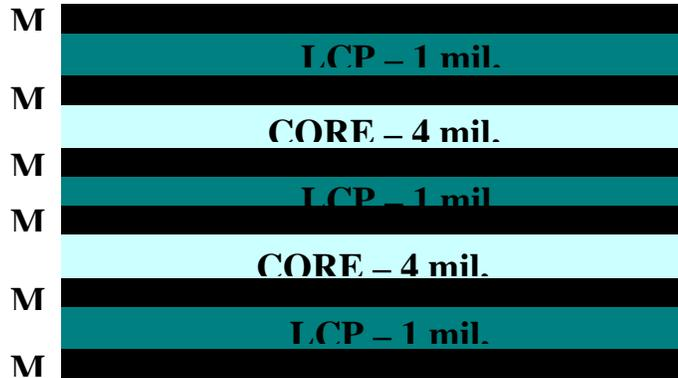
Figure 5.2. Cross-section of the three-layer LCP substrate
