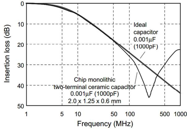
Figure 6 Insertion loss of ideal vs. non-ideal 1000pF capacitor [16]
