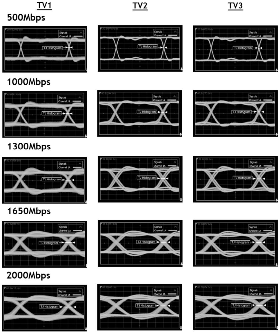
Figure 90 Eye diagrams for TV1, TV2, and TV3
