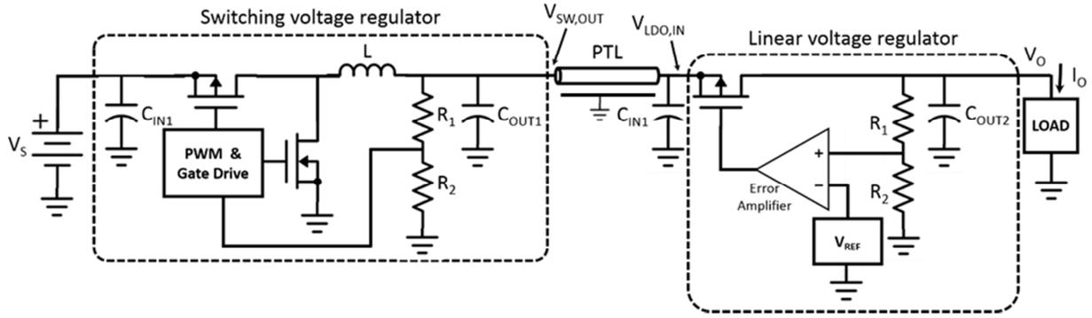
Figure 98 Power distribution network with a switching and linear regulator connected using a PTL
