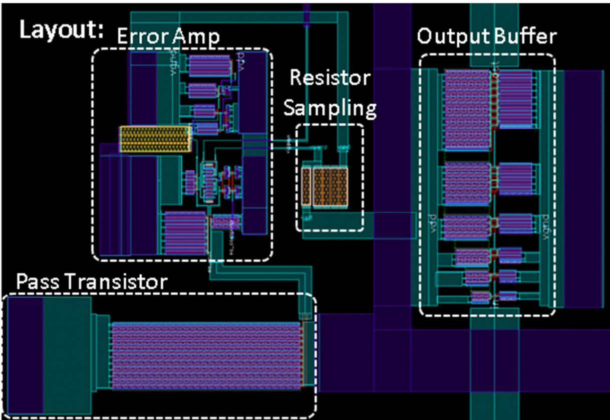
Figure 52 Layout of complete circuit
