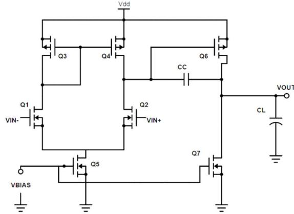
**Figure 30 Two-stage CMOS op-amp**
