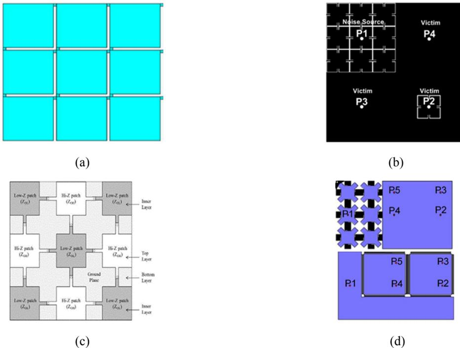
**Figure 54** Examples of EBG geometries; (a) Uniplanar EBG [21], (b) partial EBG placement [35] (c) multi-layer stepped impedance EBG [36], (d) separate EBGs on power and ground layers [37]
