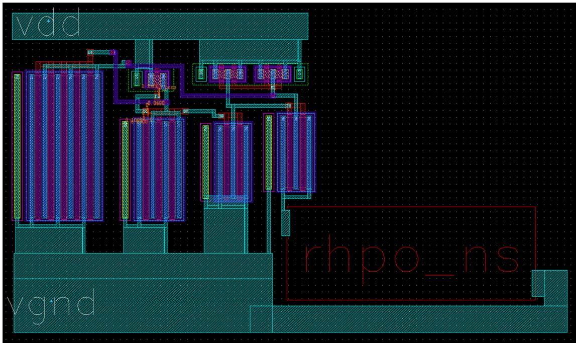
Figure 50 Layout of current reference circuit
