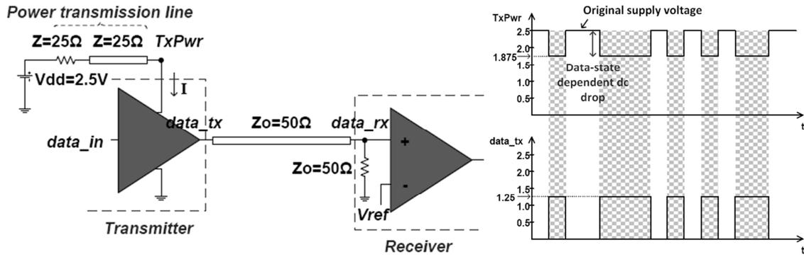
Figure 8 Single-ended signaling using a PTL (a) schematic (b) waveform showing data-dependent voltage drop on driver's supply pin[11]
