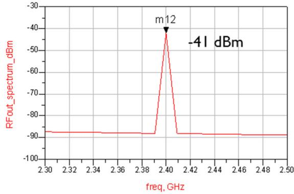
**Figure 60 Frequency spectrum of LNA output**
