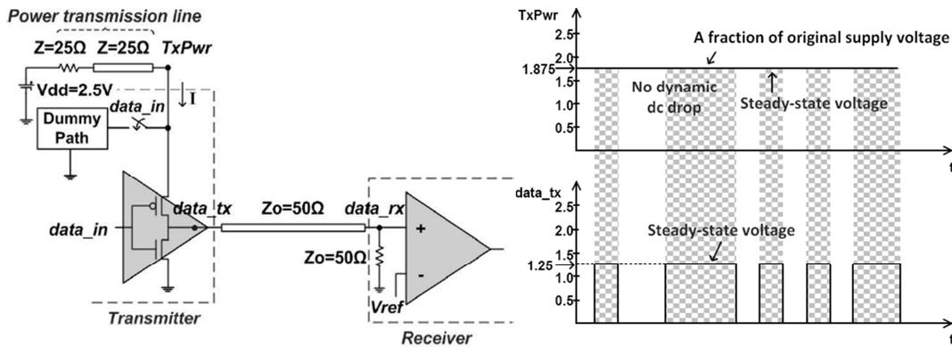
**Figure 11 Single-ended signaling using CC-PTL (a) schematic with dummy path (b) waveform with constant supply voltage [11]**
