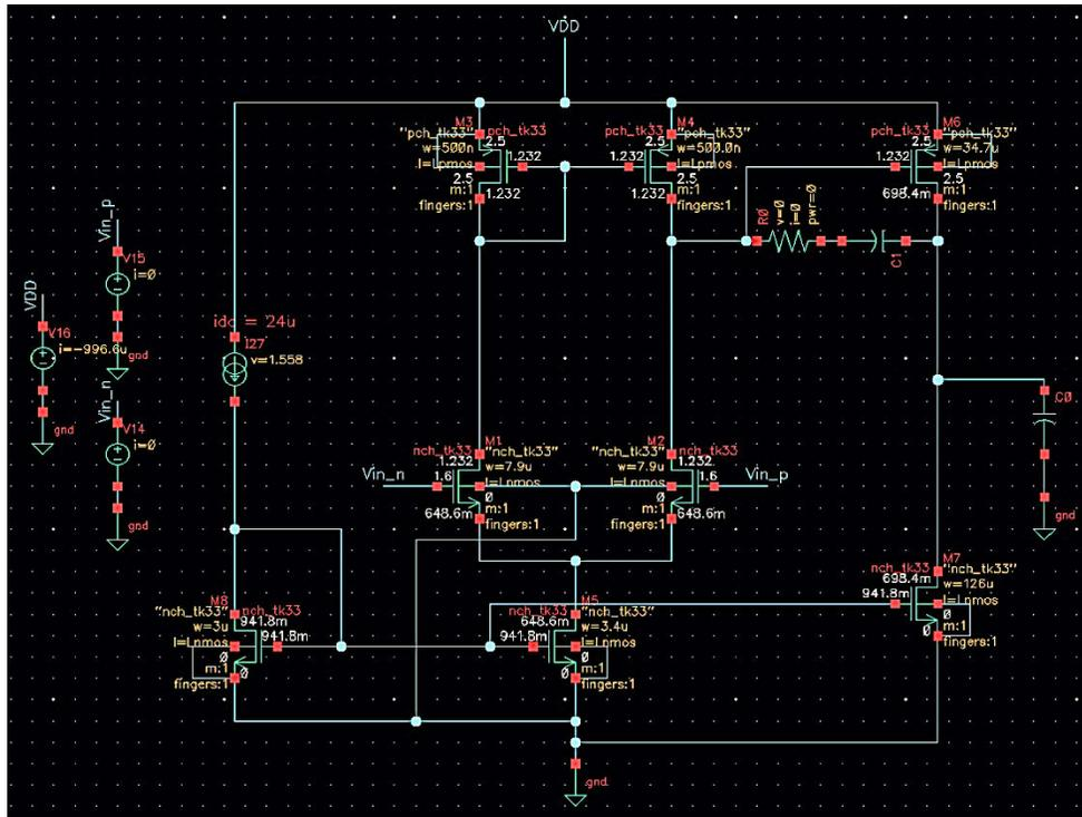
Figure 33 Error amplifier schematic in Cadence
