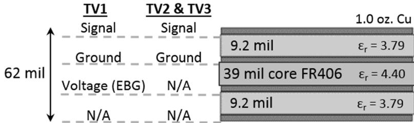
**Figure 79 Test vehicle cross-section**
