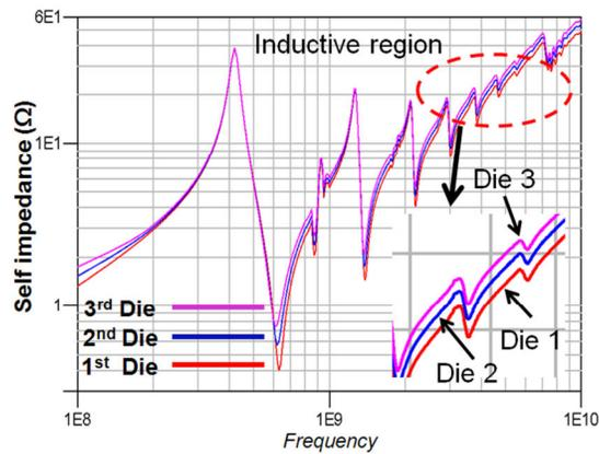
Figure 21 Impedance profile at each die, including package [8]
