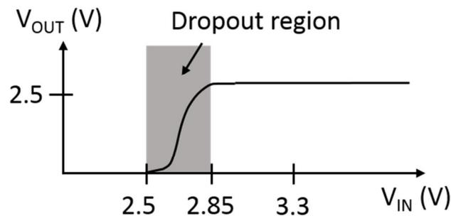
**Figure 103 Dropout voltage of LDO**
