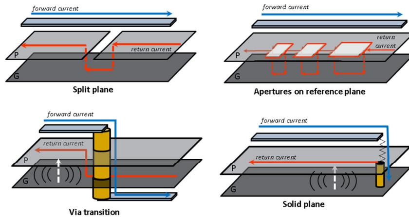
**Figure 3** Several examples showing the effect of return path discontinuities [12]
