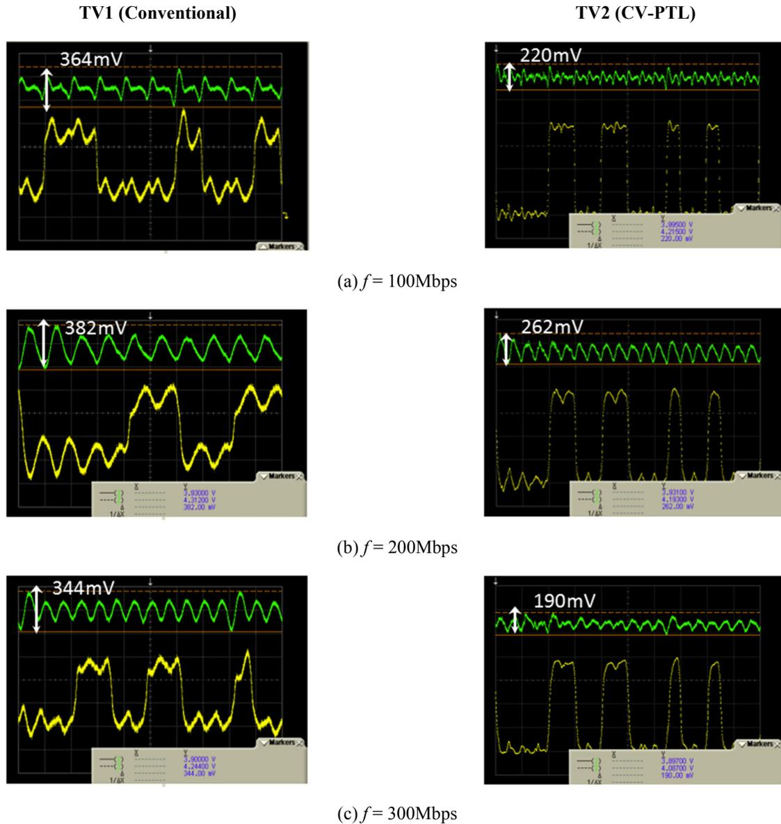
**Figure 19 Supply noise (top) and driver output voltage (bottom) for both test vehicles**
