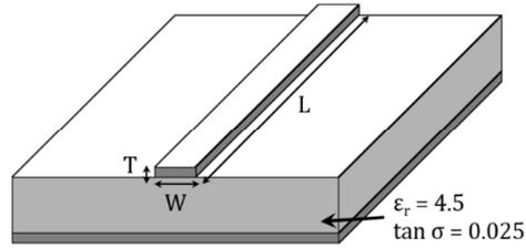
**Figure 99 Microstrip cross-section**
