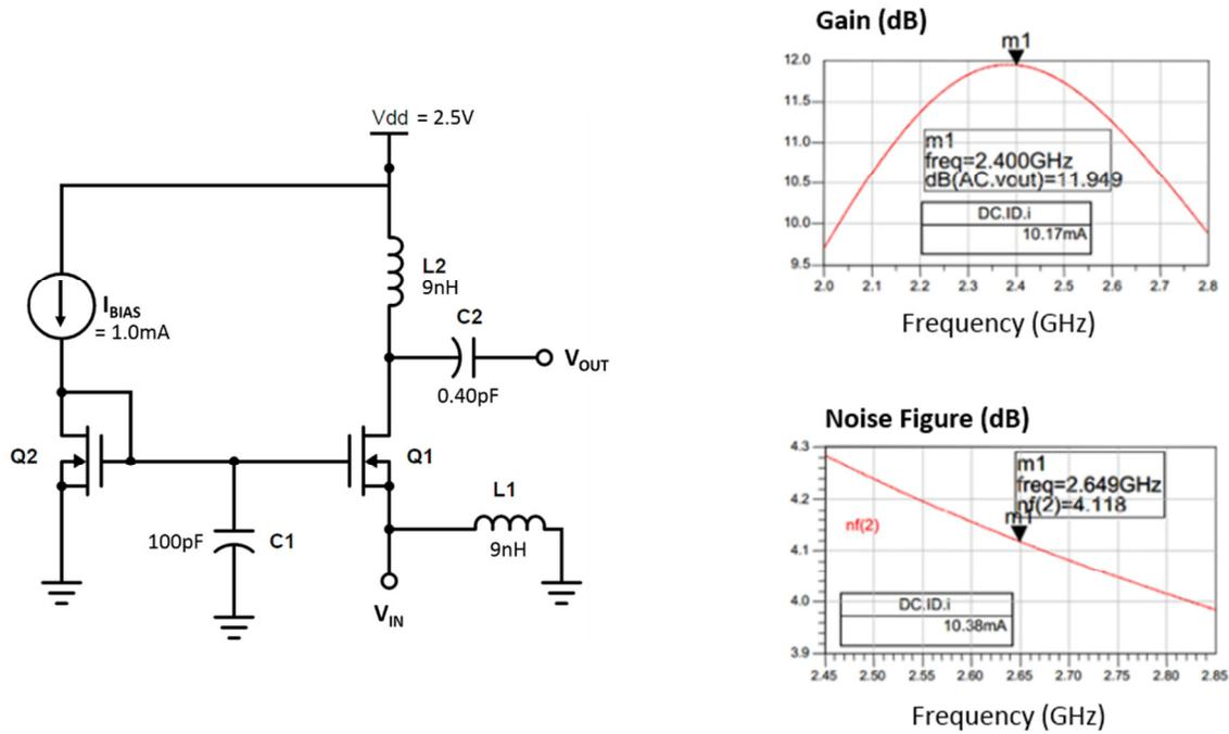
**Figure 57 RF LNA used in simulations**
