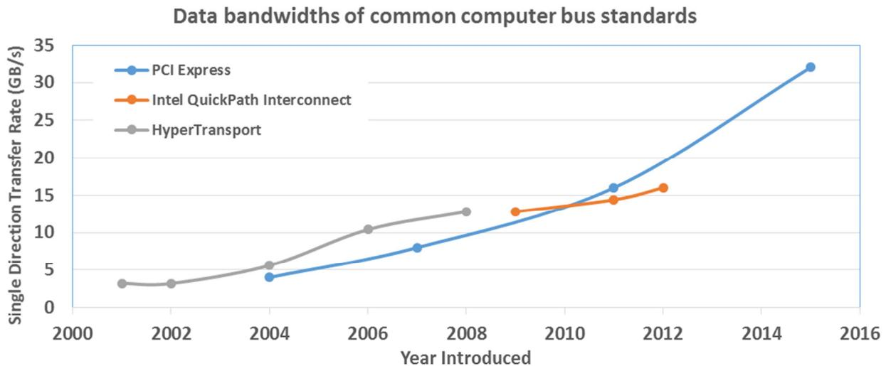
Figure 1 Increasing data rates in various commercially available I/O bus standards [1-4]
