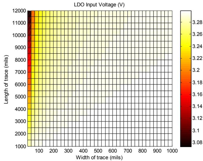
**Figure 101 LDO input voltage ( $V_{SW,OUT} = 3.3V$ ,  $V_O = 2.5V$ ,  $I_{O,Max} = 1A$ )**
