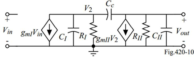
Figure 32 Small-signal approximation of 2-stage CMOS amplifier for frequency-response analysis [33]
