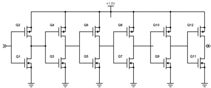
Figure 39 Buffer schematic
