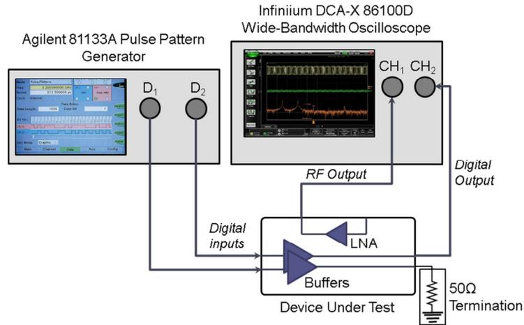
**Figure 92 Measurement setup for noise isolation measurements**
