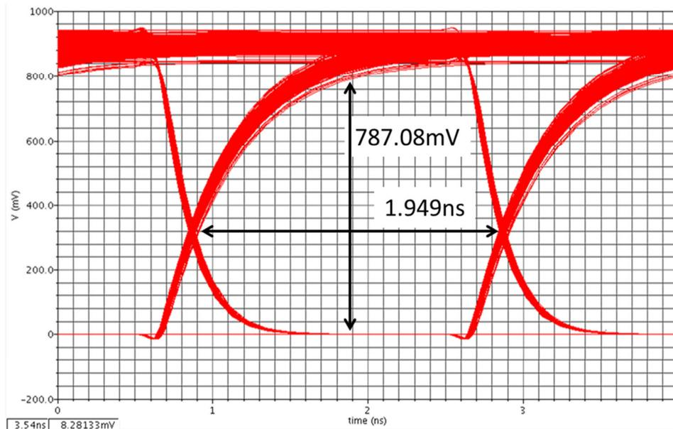
**Figure 42 Eye diagram with 500Mbps PRBS-10 input with LDO powered by PTL**
