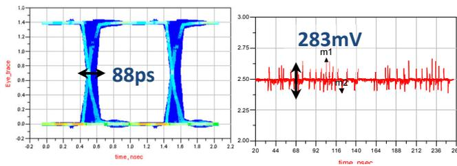
(b) Middle layer, jitter = 88ps,  $\Delta V_{DD} = 283\text{mV}$
