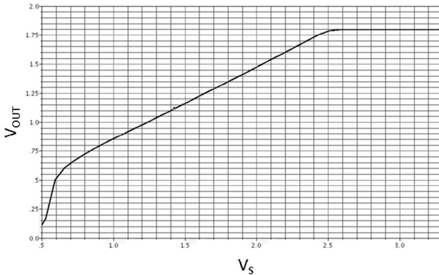
**Figure 47 Input/Output voltage characteristic of LDO**
