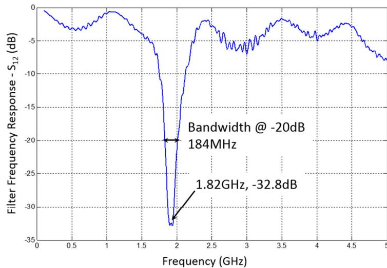
**Figure 83 Bandstop filter frequency response**
