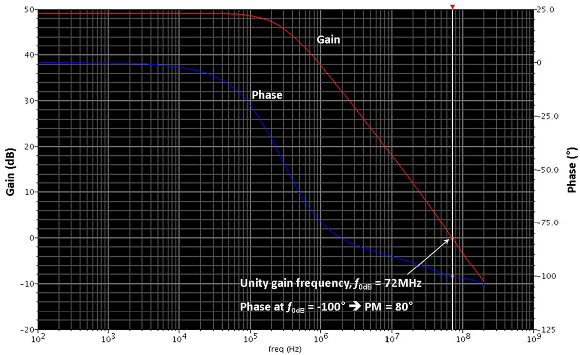
Figure 34 Frequency response of error amplifier
