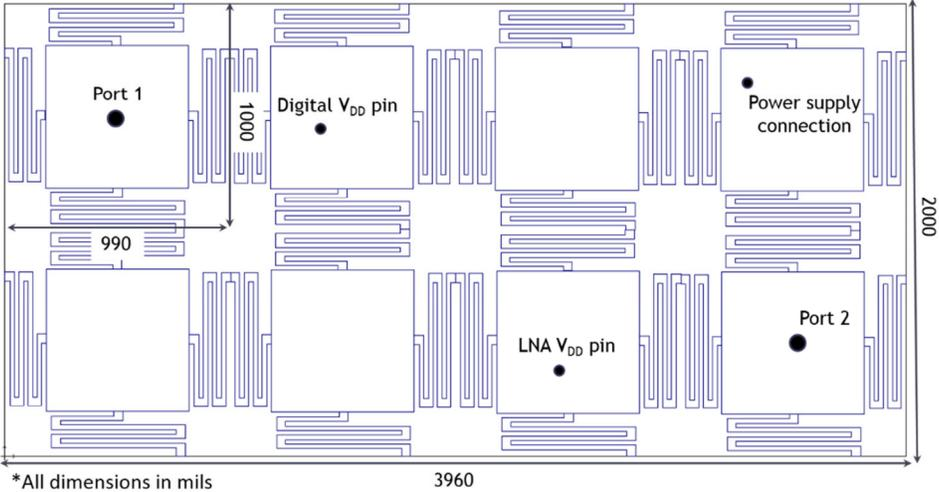
**Figure 75 Electromagnetic band gap structure**
