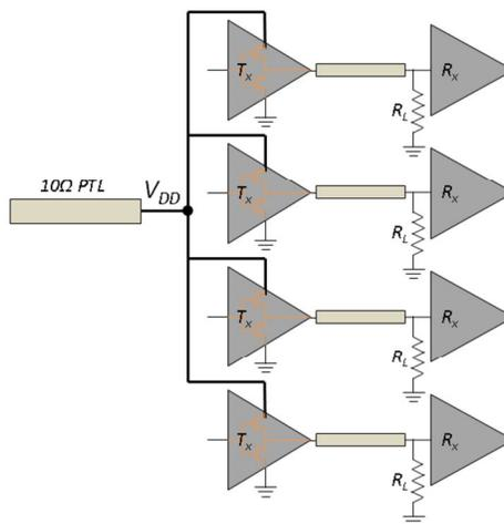
**Figure 58 Configuration of buffers and PTL in simulation**
