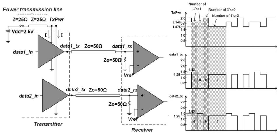
**Figure 10 PTL powering two drivers (a) schematic (b) waveform showing data-dependent voltage drop on driver's supply pin [11]**
