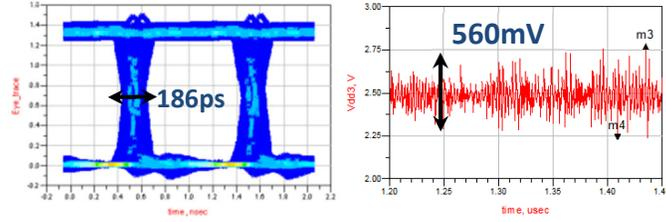
(b) Middle layer, jitter = 186ps,  $\Delta V_{DD} = 560\text{mV}$
