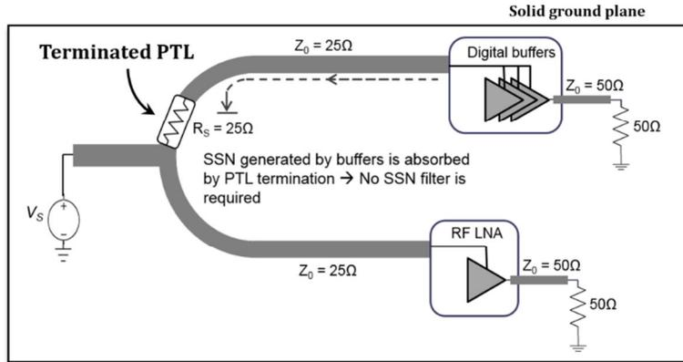
Figure 74 Mixed signal noise isolation concept using PTL termination without the filter.
