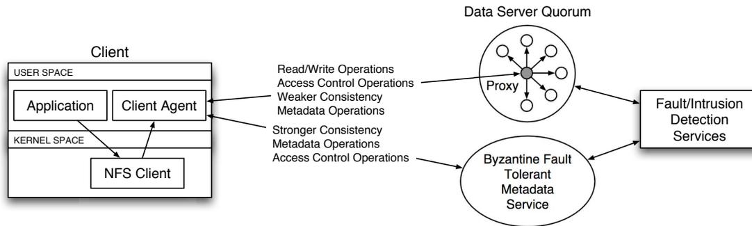
**Figure 1. Schematic overview of the file system prototype**
