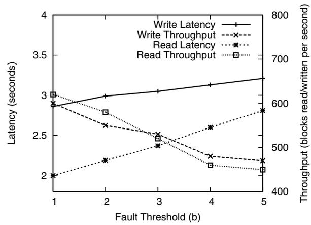
Figure 5. Agile Store base version: latency and throughput vs. fault threshold ( $n = 21$ ).
