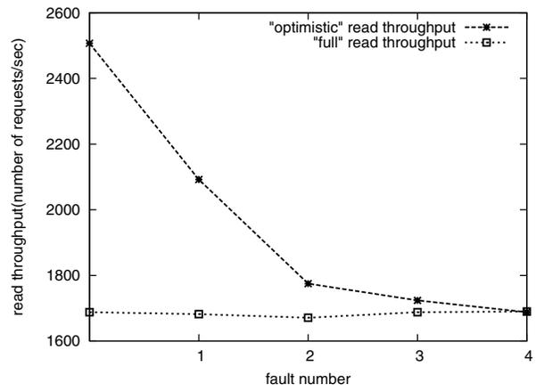
**Figure 9. Read throughput with faults (n = 17, b = 4)**
