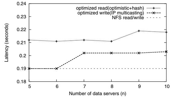
Figure 14. Comparison of the optimized version of our prototype with NFS in terms of read and write latencies on 1 MB files. The fault threshold for the prototype was kept equal to one.
