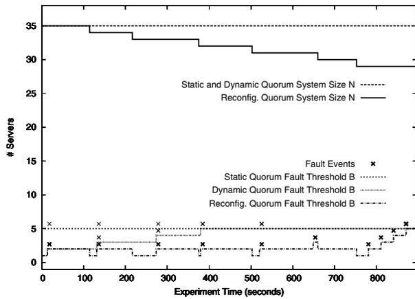
Figure 6. The variation of the number of data servers ( $n$ ) and the fault threshold ( $b$ ) when data servers become faulty over time.
