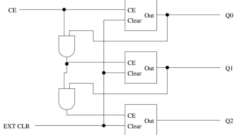
**Part C** Now use your toggle cells (in icon form) to build a divide by seven counter. This design should include a count enable  $CE$  and an active high clear  $CLR$ . Your design should clear if (A) the external clear  $CLR$  is high, or (B) the maximum output count is reached and the count enable is high. You do not need to draw in the clock signals.
